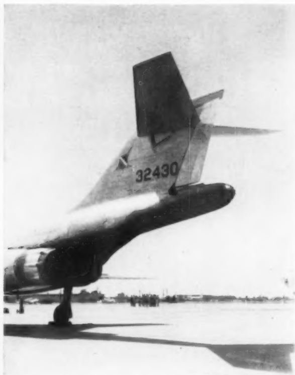
TWIN TURBOJETS of the Voodoo exhaust below the tail supporting structure. Fairing between engines and under forward part of boom is titanium structure to take the heat, blast and corrosive effects of the tailpipe and maintain strength. Note large travel of the high-mounted slab tail.
